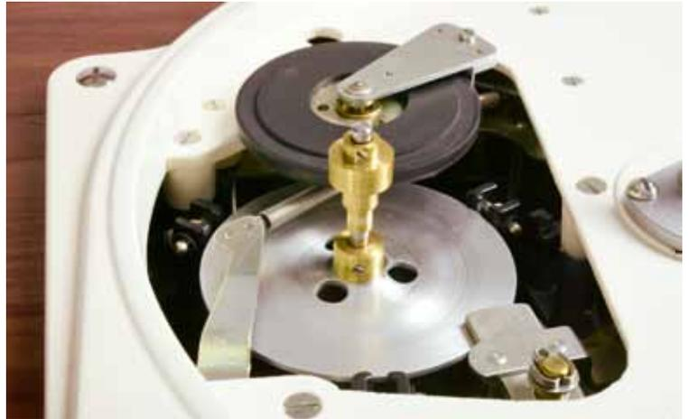
A stepped shaft performs the speed changeover purely mechanically; the friction wheel transmits frictionally to the inner rim of the platter
